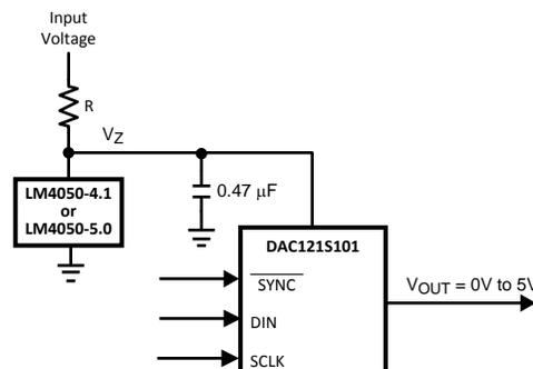
Figure 42. The LM4050 as a power supply
