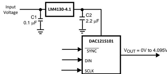
Figure 41. The LM4130 as a power supply
